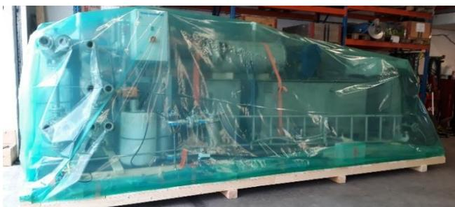
Since a few days, an A.H.T. syngas power plant with a nominal output of 150 kW<sub>el</sub> is on its way to Southeast Asia. This system, equipped with an ignition oil system for the use with biodiesel, is the first stage for a 5 MW installation. The engineering for this plant complex had been ordered and
